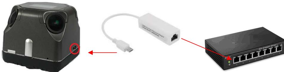
**1-4.** After connection, the OLED screen will show the IP.
